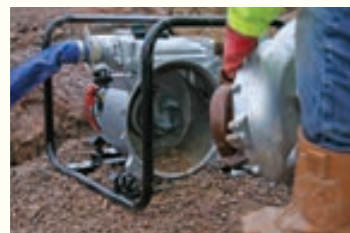
The removable inspection cover allows quick simple access
